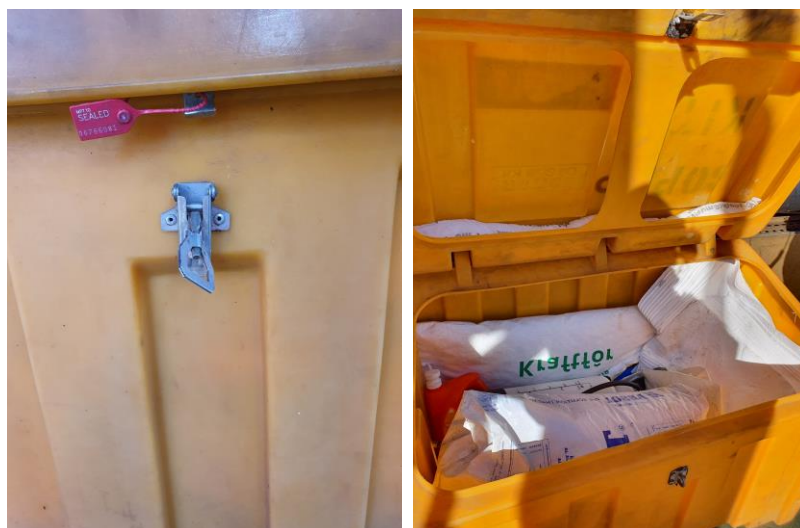
Figure 4-9: Missing sealing (to the left) and inventory list and lacking equipment (right)
