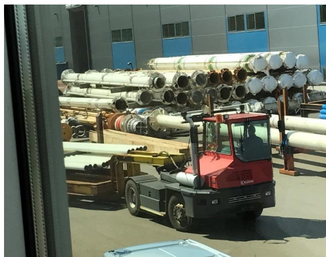
Figure 4 PSW Inhouse Tractor for towing capping stack flatbed trailer
