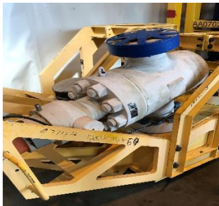
Figure 10 Flowline frames and valves for flowing well
