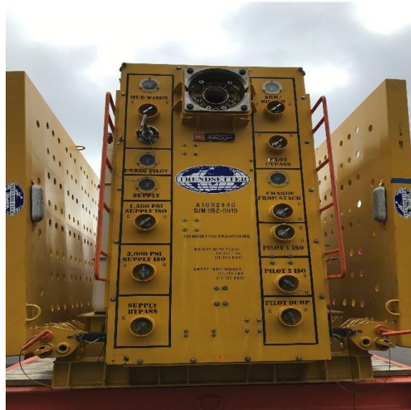
Figure 6 SAM Modules designed for both capping stack and BOP Intervention
