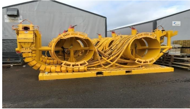
Figure 7 Cobra Head and Flying Lead for BOP Intervention
