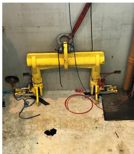
Figure 12 Spreader bar for deployment of stack by wire from vessel
