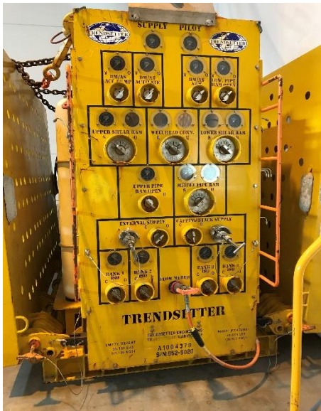
Figure 6 SAM Modules designed for both capping stack and BOP Intervention
